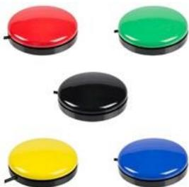
Switches work particularly well with 'cause and effect' software and programs that require simple choices but can also be used to fully control a computer. A small switch interface box is needed to connect a switch to a computer, although some 'all-in-one' and wireless options are now available.
